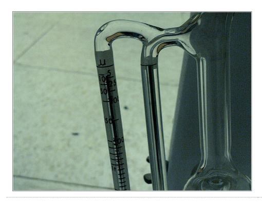
were able to obtain a 5 micron (Hg) or 5 mtorr vacuum as measured using a McLeod gauge. Awesome!
