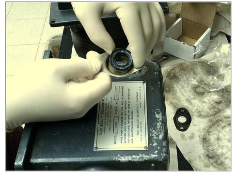
picture of the oil case with the gas ballast seal removed.
