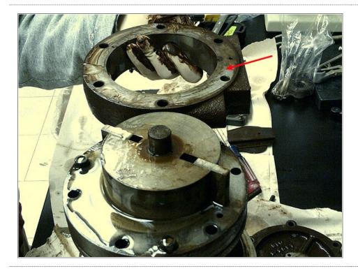
Step 19 Exhaust stage disassembly
