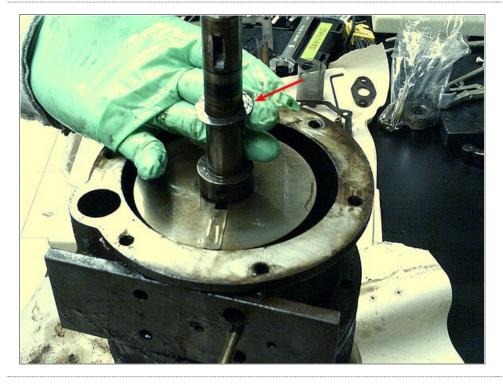
Step 18 Exhaust stage disassembly
