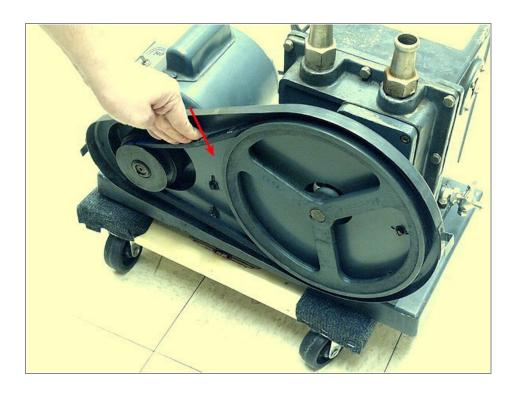
ratio, and thus the belt tension, using a percussive method. We loosened the AC motor bolts, and used a rubber mallet to make minor displacements to the motor position. You should avoid making major adjustments to the motor position unless you have force gauge to properly set the V-belt tension.
